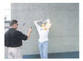
The PSC splatter stream samples, serial numbers 091711, 082811, did not ignite nor did they produce any visible flame or significant heat changes on the thermal measuring equipment.
